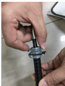
Remove the ring by turning counterclockwise
